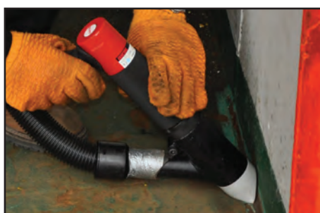
CONTAINMENT OF MATERIAL AT SOURCE
